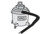
Shop vacuum for cleaning out dust and debris from cracks and spalls.
