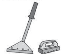
Sharp scraper for shaving off cured material and sanding brick for smoothing and blending repairs.
